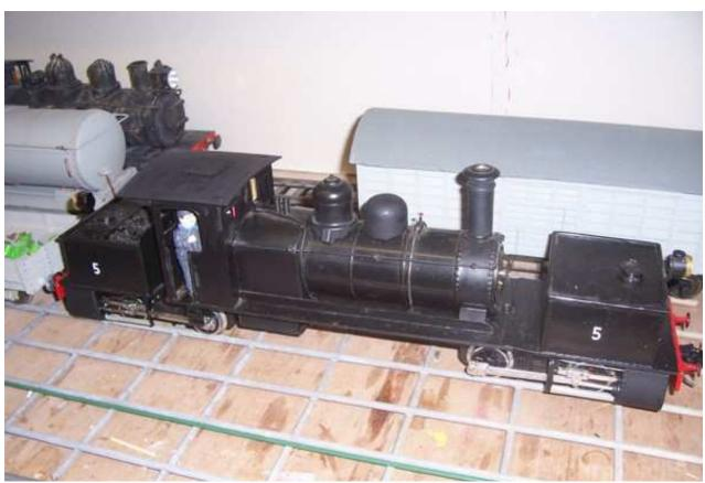
A Bigger Chimney, Steam dome, addition of a Sand dome and an enlarged Cab roof with rear overhang were all added to create this unique freelance Garratt in 1/24<sup>th</sup> scale for the BTR Locomotive roster.
